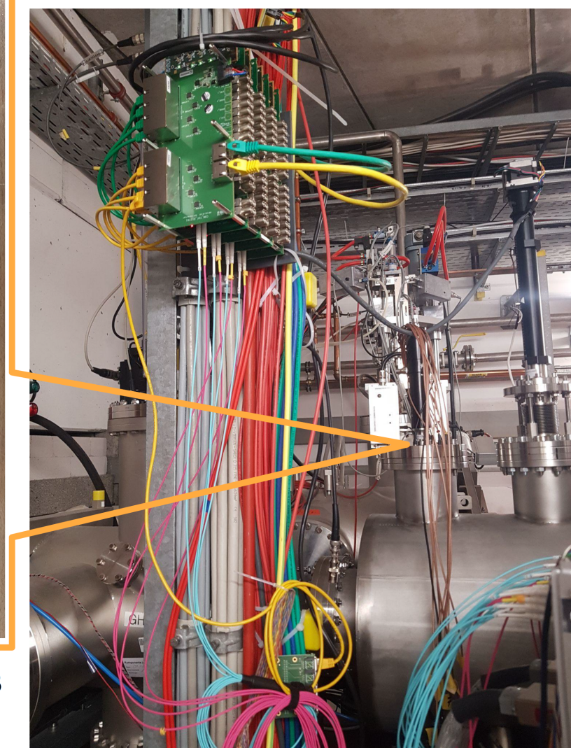
Diamond interface PCB with pneumatic drive
