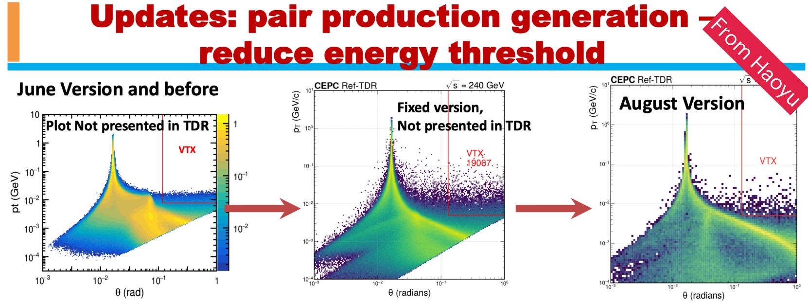
Decrease the threshold on electron/position output from 5 MeV(the built-in value) to 0.511 MeV, results shown at 50 MW Higgs
