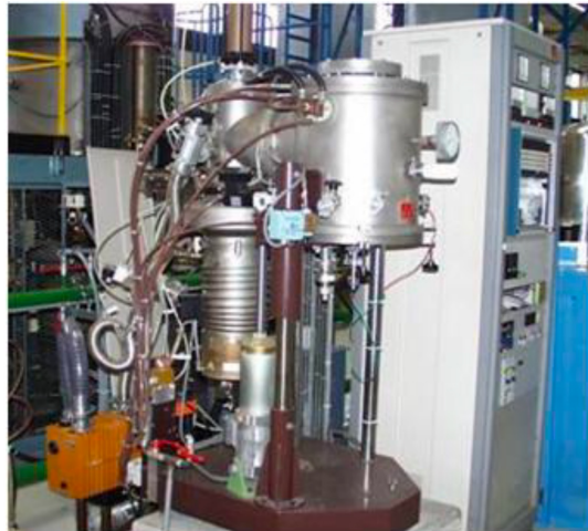
VAS furnace. Maximum temperature 1600°C, used for small sample
