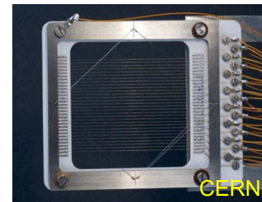
wire welded to ceramic plate
