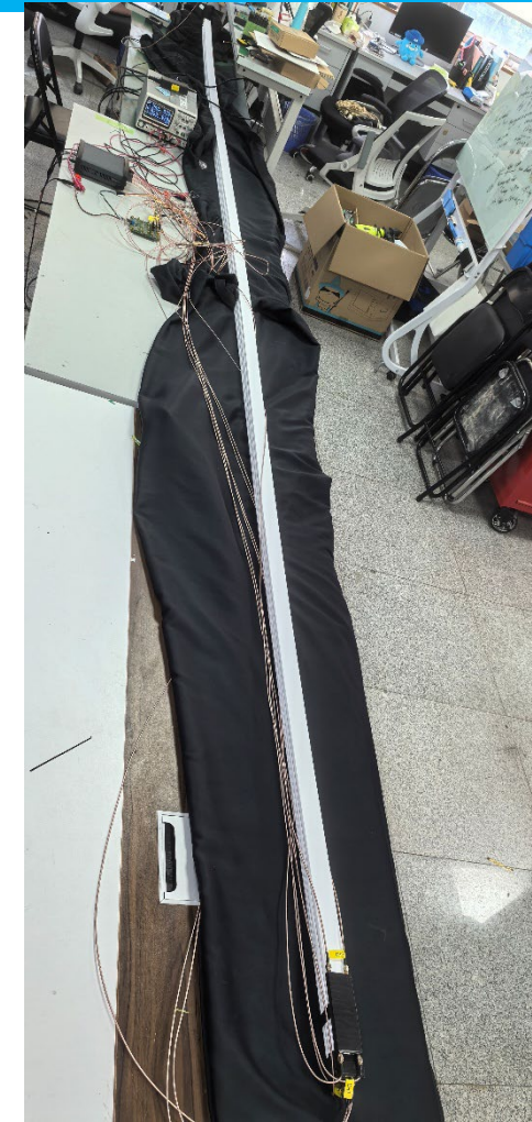
5m PSU prototypes under CR tests.
