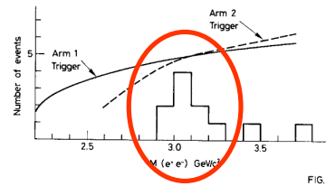
Fig. 2. Invariant mass distribution for the observed e^+e^- pairs. The curves represent the shapes of the acceptance, as a function of the e^+e^- invariant mass value, for the Arm 1 and Arm 2 triggers, respectively.
