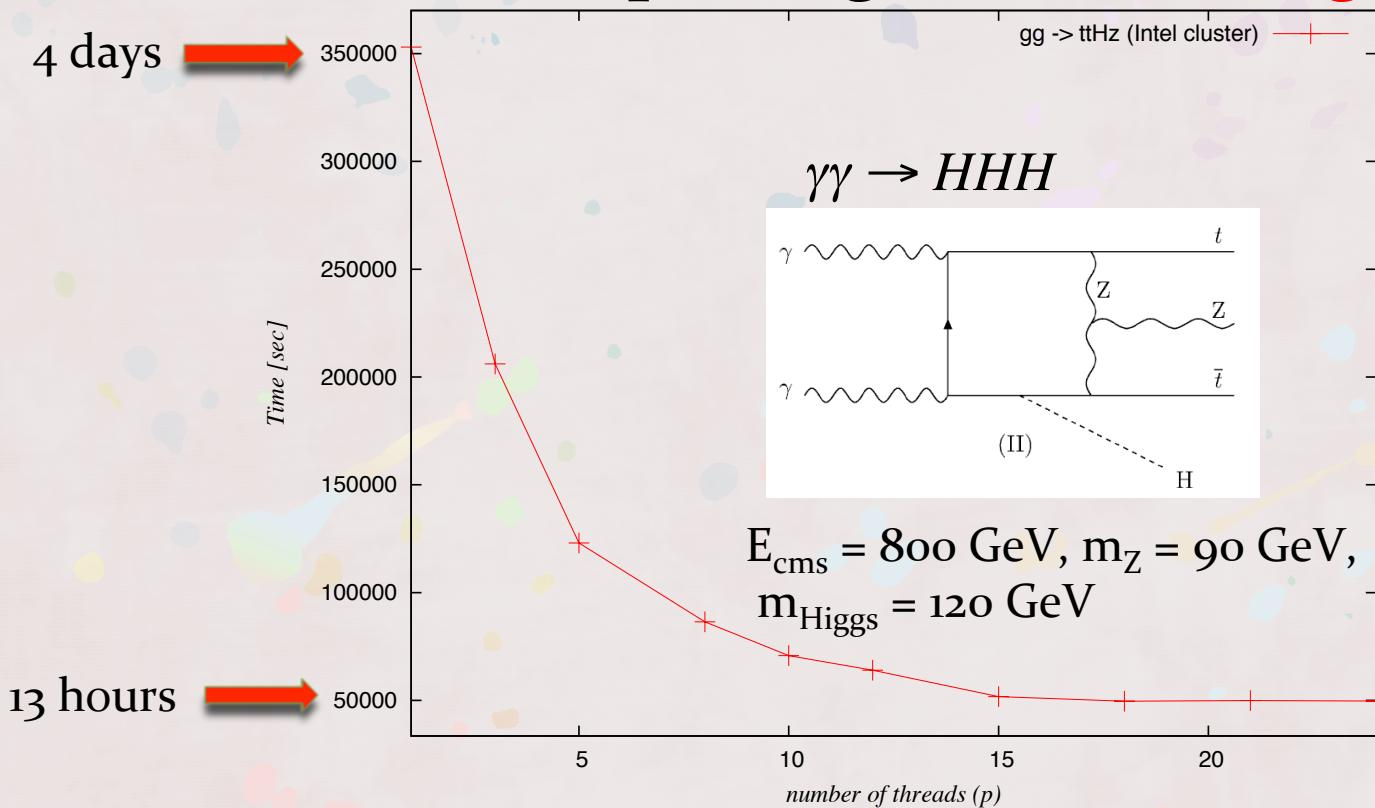
Timing plot on WMU cluster (Xeon E5-2670, 16 cores /node)
