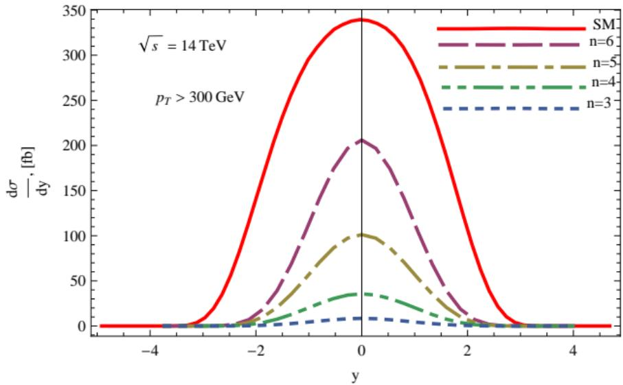
$pp \rightarrow \text{jet} + Z_{\text{bulk}}^0 (\gamma_{\text{bulk}})$  (dashed lines) The jet transverse momentum cut is  $p_T > 300 \text{ GeV}$ . SM background is  $pp \rightarrow \text{jet} + \nu\bar{\nu}$  (solid line). At the LHC energy  $\sqrt{s} = 14 \text{ TeV}$ . The main background contribution comes from  $300 \text{ GeV} < p_T < 800 \text{ GeV}$
