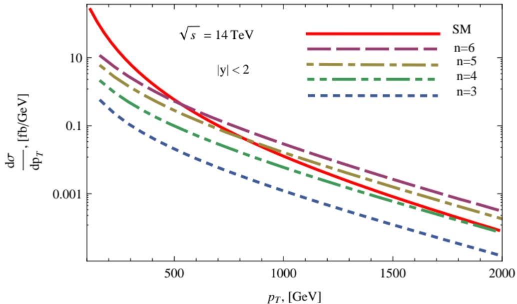
$pp \rightarrow \text{jet} + Z_{\text{bulk}}^0(\gamma_{\text{bulk}})$  (dashed lines). The jet rapidity cut is  $|y| < 2$ . SM background -  $pp \rightarrow \text{jet} + \nu\bar{\nu}$  (solid line). At the LHC energy  $\sqrt{s} = 14 \text{ TeV}$ . Signal dominates:  $p_T > 500 \text{ GeV}$  for  $n = 6$ ,  $p_T > 800 \text{ GeV}$  for  $n = 5$
