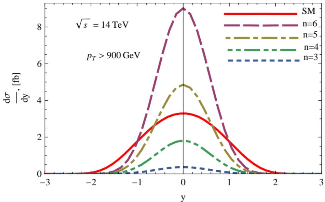
Diff. cross section of  $pp \rightarrow \text{jet} + Z_{\text{bulk}}^0(\gamma_{\text{bulk}})$  (dashed lines) The jet transverse momentum cut is  $p_T > 900 \text{ GeV}$ . SM background is  $pp \rightarrow \text{jet} + \nu\bar{\nu}$  (solid line). The center-of-mass energy of incoming protons is  $\sqrt{s} = 14 \text{ TeV}$ .
