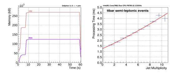
Figure 1. Left: memory usage as function of time after the program start. Right: processing time per event as function of jet multiplicity on inclusive  $t\bar{t}$  events.
