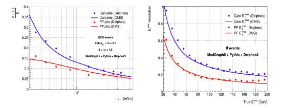
Figure 2. Comparison of the performance achieved with DELPHES fast-simulation tool against the CMS experiment full-simulation. Left: Jet energy resolution as a function of the jet  $p_T$  in QCD events. Right: Missing transverse energy resolution as a function a of the true event missing transverse energy in top-pair events.
