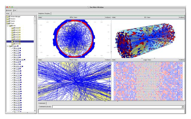
**Figure 3.** QCD event with 50 pile-up interactions shown with the DELPHES event display based on the ROOTEVE libraries [12]. Transverse view (top left), longitudinal view (bottom left), 3D view (top right),  $(\eta, \phi)$  view (bottom right).
