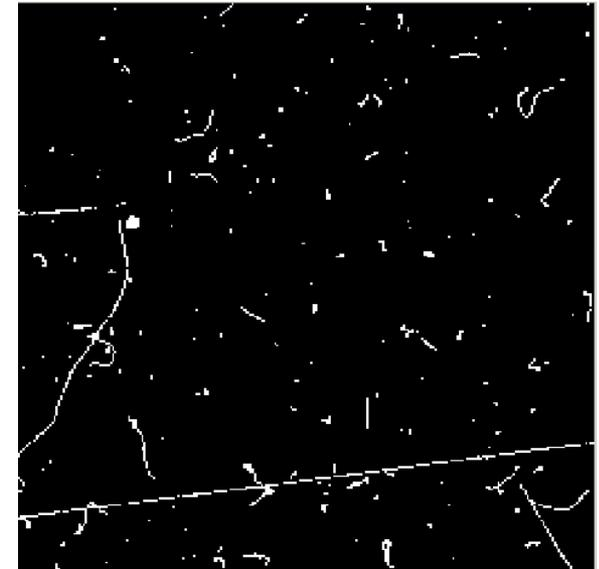
Functions as an active nuclear emulsion, allowing the visualization of the individual tracks created as the different incident particles traverse the detector.
