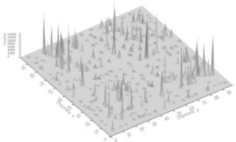
Spectrum after boosted Gold deconvolution (50 iterations repeated 20 times).
