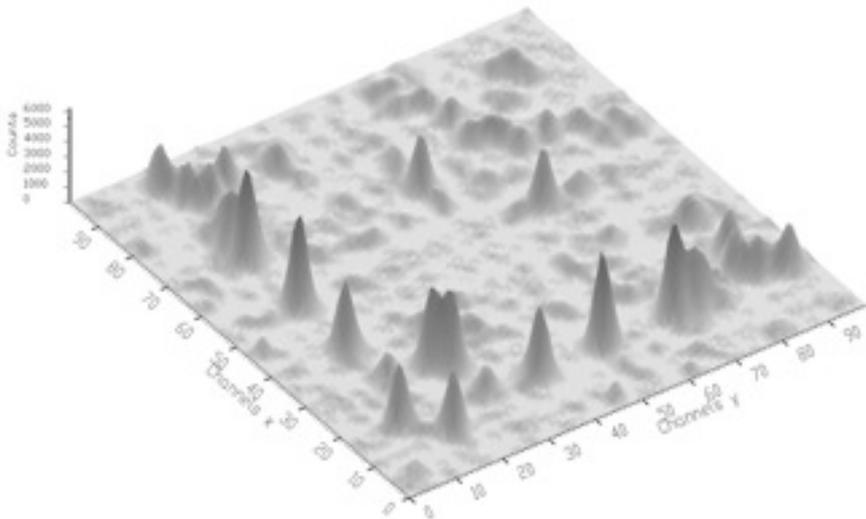
Experimental gamma-gamma-ray spectrum (after background elimination).
