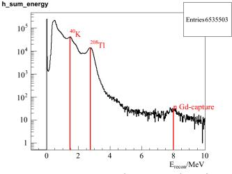
Fig. 2 Reconstructed energy distribution for all triggers in one AD
