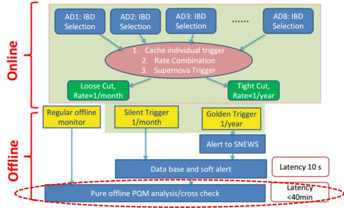
Thanks Hanyu WEI for providing me the diagram. More details in his talk 'Supernova Trigger in the Daya Bay Reactor Neutrino Experiment' in Track 2.
