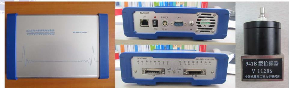
Vibrometers: 3 by 941B vibration pickup;
