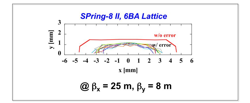
Injection to a Ring with a Small Dynamic Aperture
