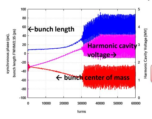
Bunch center of mass and bunch length oscillate above 2.7MV.
