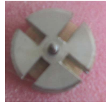
circle WLS fiber in the mold
