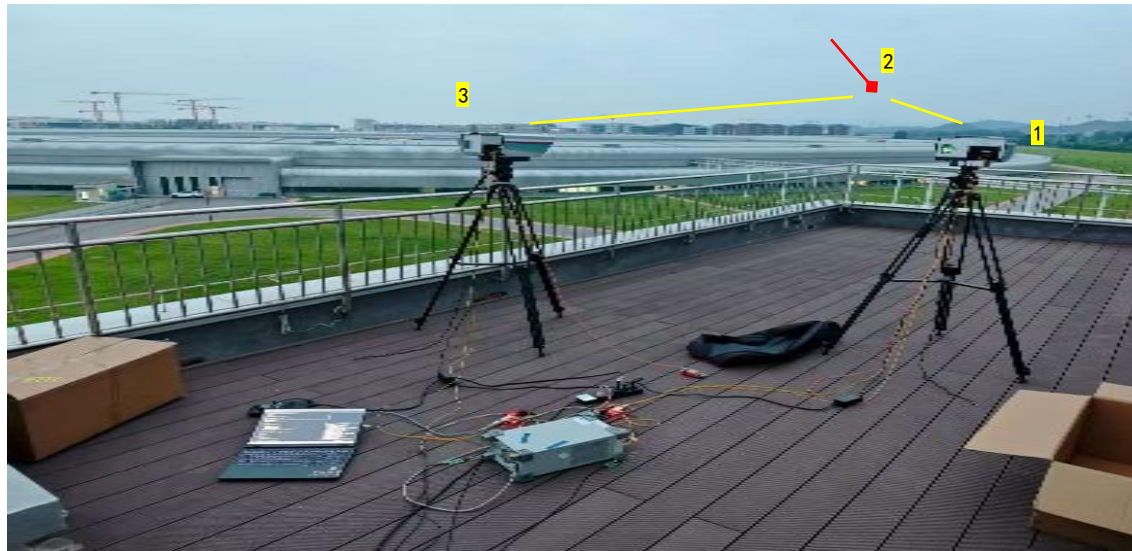
500 m Round-Trip Laser Wireless Transmission Test in HEPS campus
