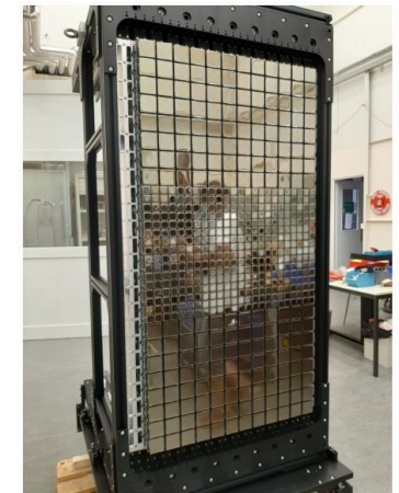
Multi-anode metal-channel dynode PMT (LHCb RUN3)
