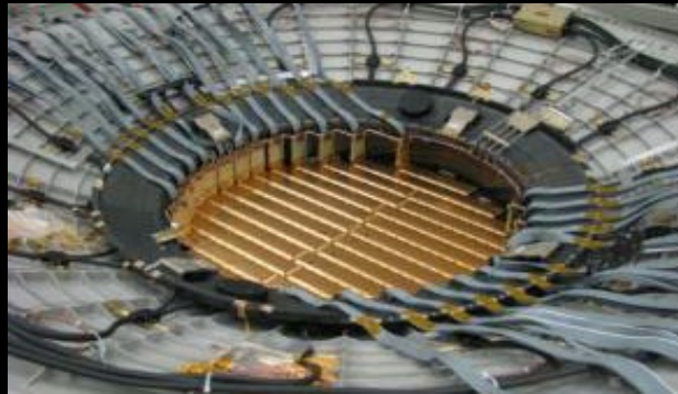
Ring Imaging Cerenkov (RICH) measure Z, E
