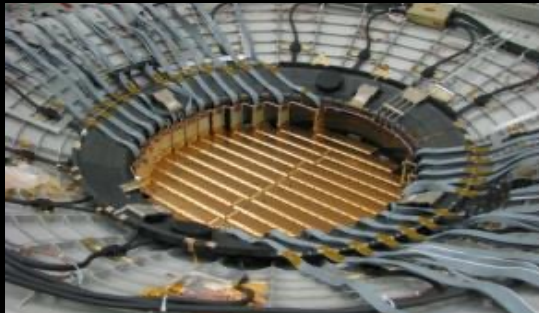
Ring Imaging Cerenkov (RICH) measure Z , E
