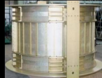
Anticoincidence Counters (ACC) reject particles from the side
