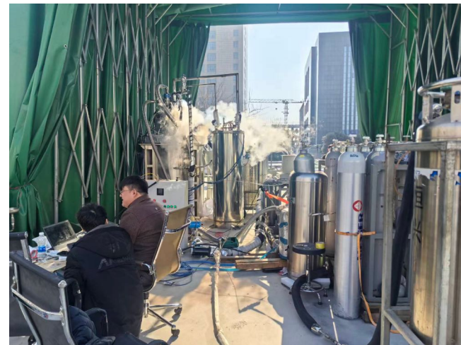
High-power cooling recovery R&D System Target: 20kW cooling power for 850kg/h circulation
