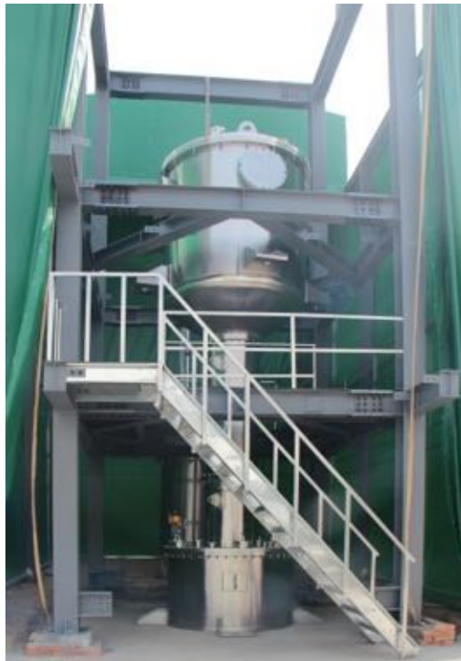
High-power cooling recovery R&D System Target: 20kW cooling power for 850kg/h circulation
