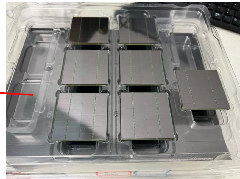
Epoxy resin (thickness: 0.65 \pm 0.2 ) 32x MPPC chip : effective photosensitive area 12.0(X) \times 6.0(Y)
