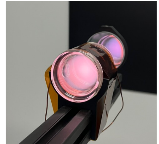
1 mbar ^3\text{He} glass cell produced at CSNS
