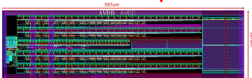
The data phase control module (90%)
