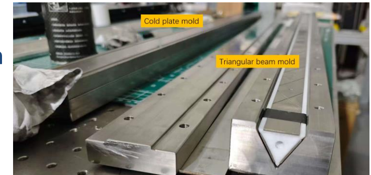
Mold for CF beam and cold plate
