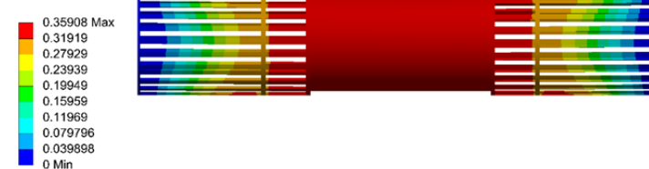
ITK deformation: 0.36mm (fix to TPC endplate)→0.23mm (fix to TPC inner cylinder)
