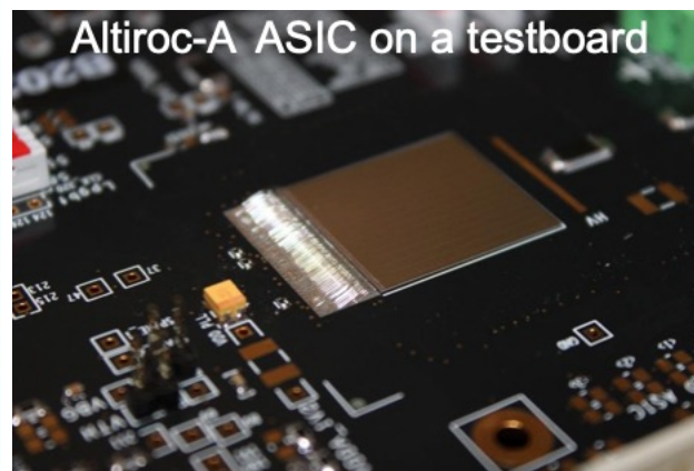
ASIC chip testing in test board
