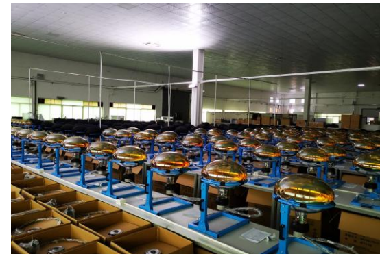
PMT potting workstation
