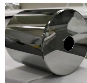
ICPC: Inverted Coaxial Point Contact Φ 80 × 80 mm, mass ~ 2 kg
