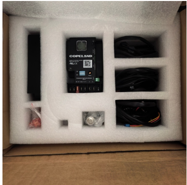
Electronic expansion valve (EEV) driver
