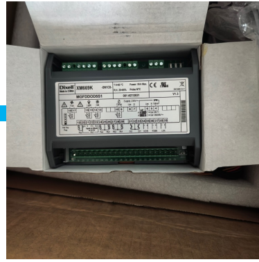
Expansion valve driver
