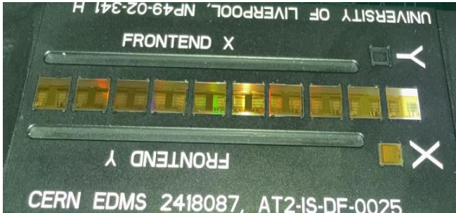
HCC loading into Jig
