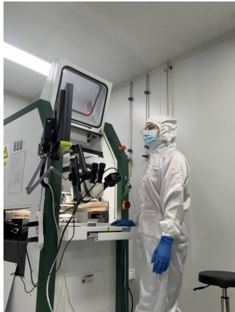
Wire Bonding at IHEP
