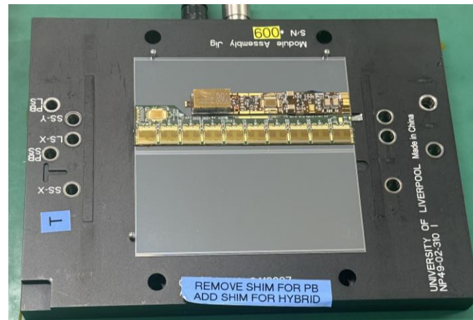
Module in Assembly Jig
