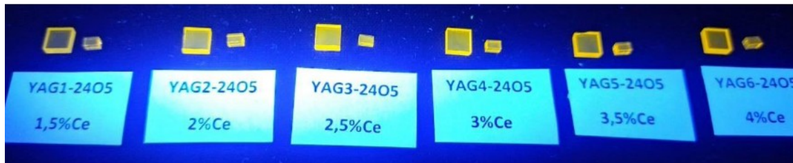
ISMA YAG:Ce samples (1.5–4 % Ce): no Ir crucible needed, but ~100 ns; co-doping aims at ~20 ns. Work supported by the European TWIN project TWISMA (GA: 101078960)
