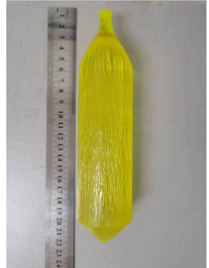
A GAGG:Ce ingot grown by SIPAT
