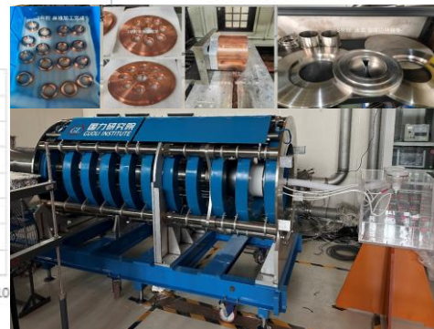
Klystron No. 3 (MBI) Efficiency 80.5% To be completed in 2026
