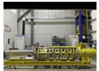
Klystron No. 2 Efficiency 77% (2021)
