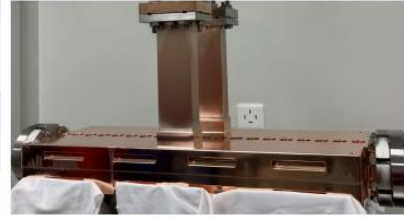
Type I: Aperture diameter 5mm, Length 0.5m
