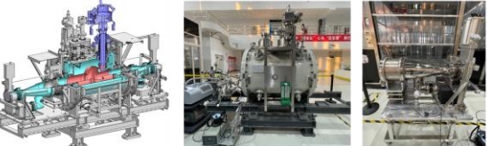
500 MHz KEKB-type single-cell SC cavity module
