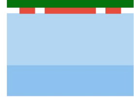
③ Thermal Oxidation + SiO 2 Deposition
