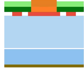
⑨ Substrate Thinning + Backside Metal
