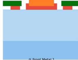
⑤ Front Metal 1 (Ti/Al/Ti/Ni)
