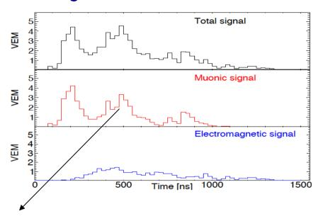
Muons stand above smooth electromagnetic component in FADC traces
