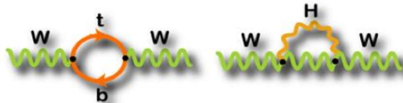
Precision measurements of  $M_W$  and  $M_t$  constrain SM Higgs mass.
