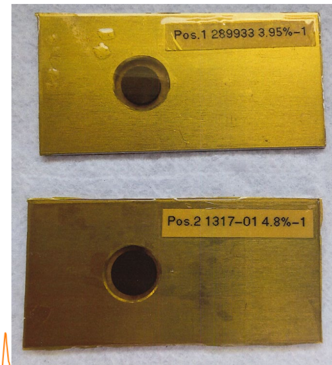
Nuclear fuel pellet slabs ready for irradiation at MIXE. Each slab is about 9mm diameter and weighs 0.5g.
