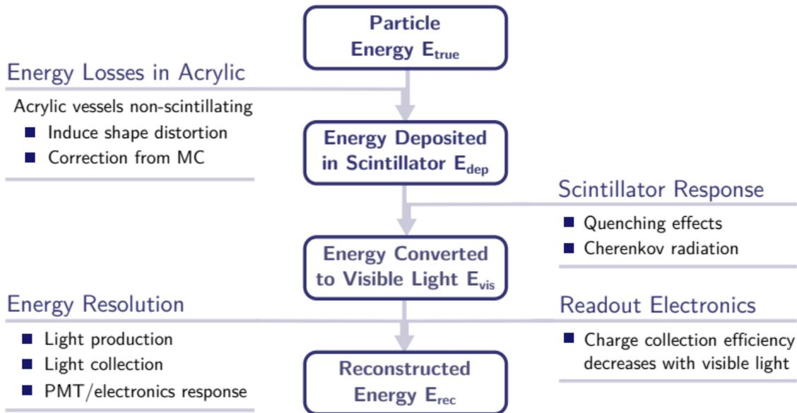
Model maps reconstructed energy  $E_{rec}$  to true kinetic energy  $E_{true}$
