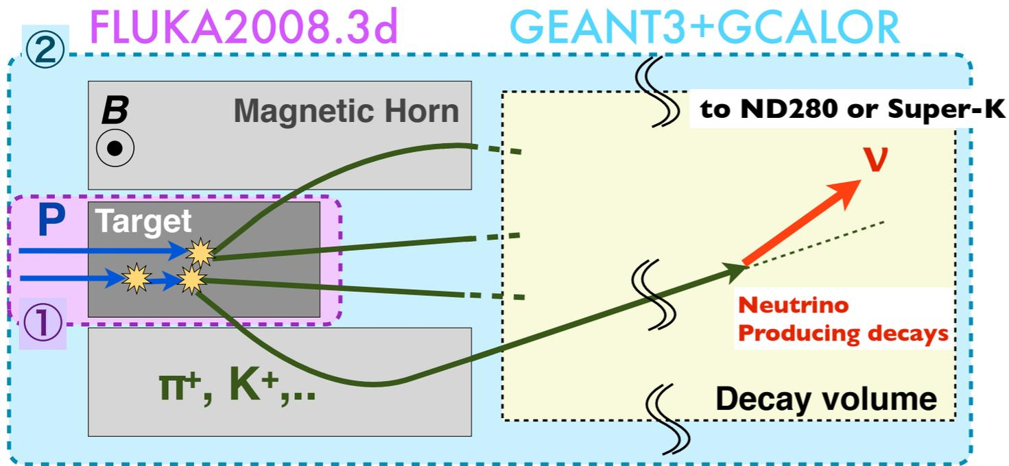
Use NA61/SHINE data for  $\pi, K$  production to tune simulation
