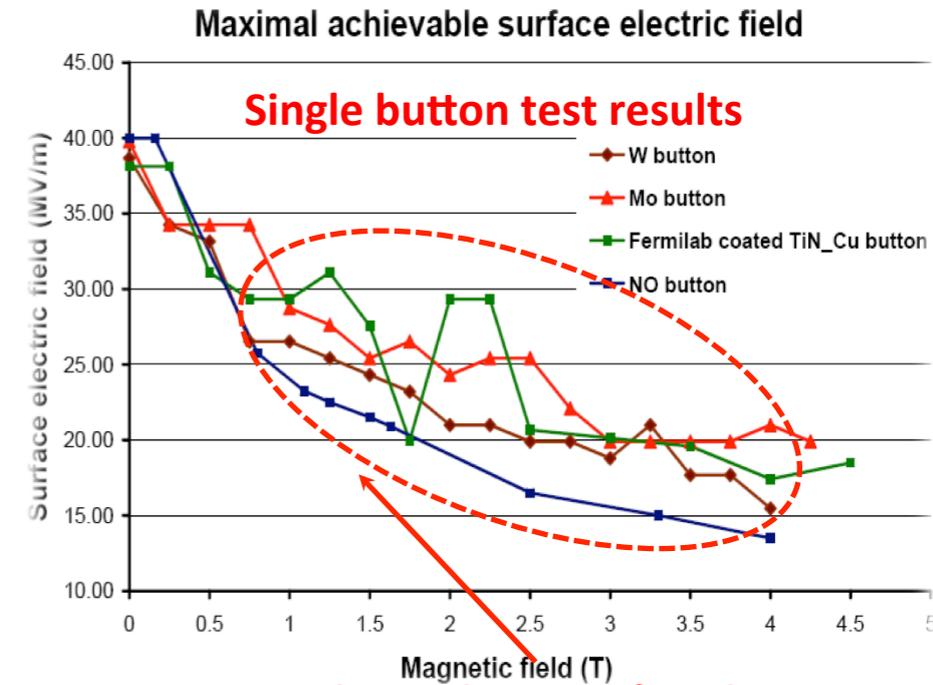
Scatter in data is due to surface damage on the iris and the coupling slot
