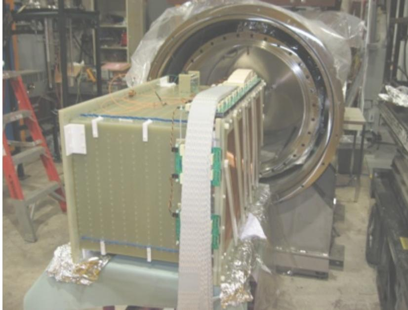
The TPC, about to enter the inner cryostat
