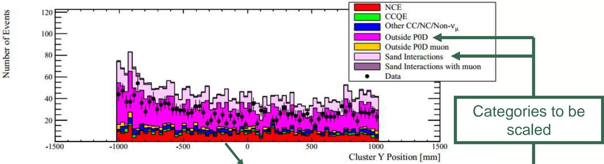
Fit for scaling factor for Outside P0D + Sand interaction without muons. Vary all other event categories independently with normalization errors:  $S_{external} = 0.396 \pm 0.096$
