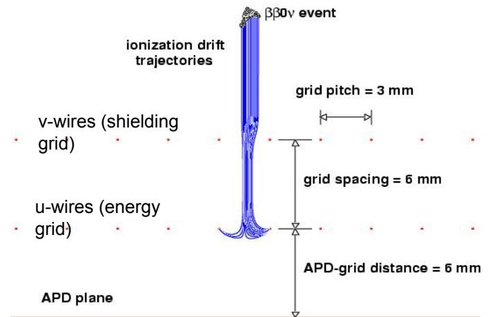
Simulation of Charge Drift
