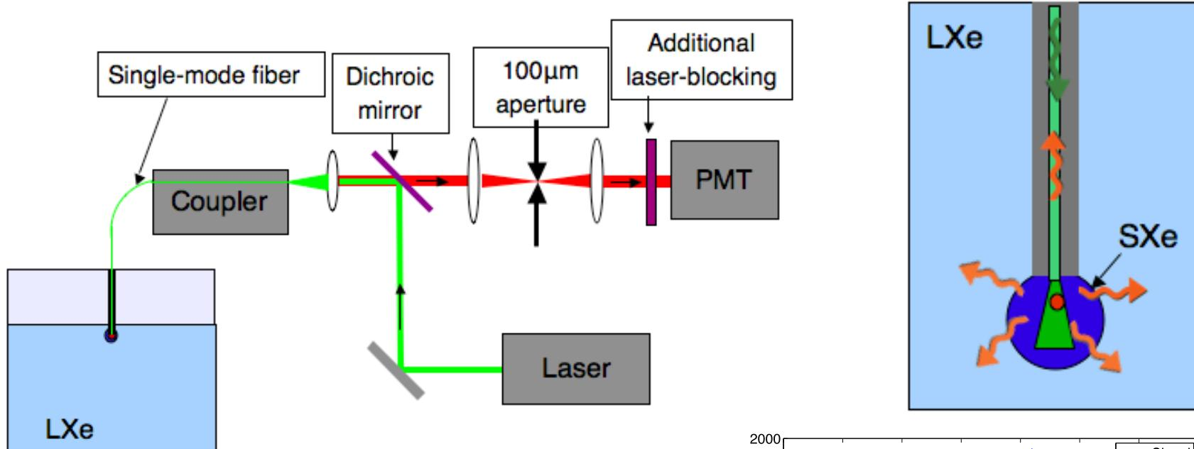
Laser light delivered by fiber to single Ba atom or ion in solid xenon. Fluorescence collected back up the fiber and detected by PMT or APD.
