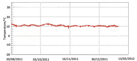
Figure 27: Temperature stability of Tracker Planes 5 and 6 over 4 months.
