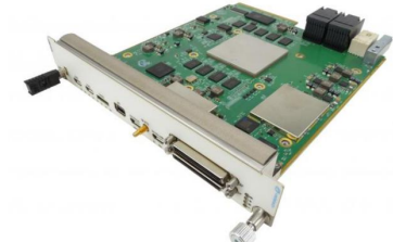
AMC576 RF-SoC 16 ADC (12-bit @ 2 GSPS) 16 DAC (14-bit @ 6.4 GSPS)
