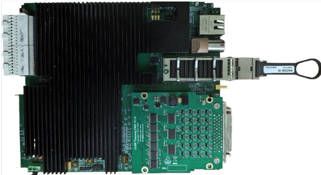
The carrier card: converters and clocking feed the FPGA; AMC connector at the rear edge
