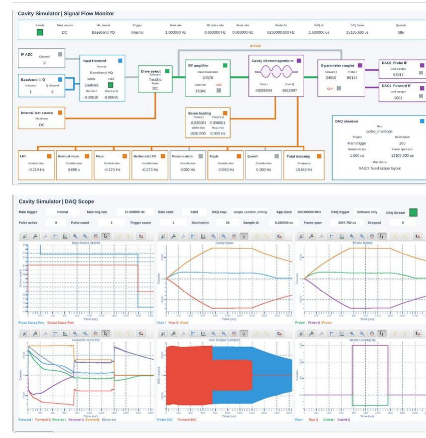
EPICS signal-flow monitor (top) and DAQ scope (bottom)
