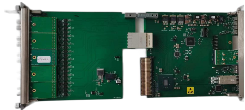
Figure The Rear-Transition Module for trigger distribution
