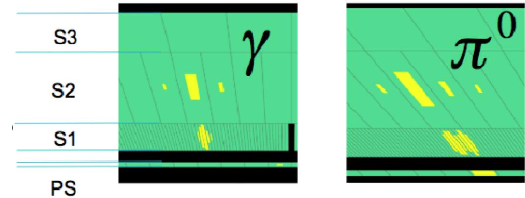
The ATLAS calorimeters are finely segmented and can effectively distinguish between isolated photons and backgrounds like  $\pi^0 \rightarrow \gamma\gamma$
