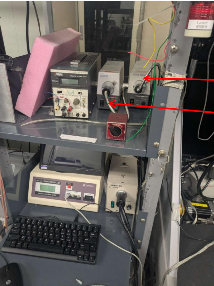
Focusing optical path tube (spot size down to 2 microns)
