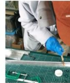
Applying release agent
