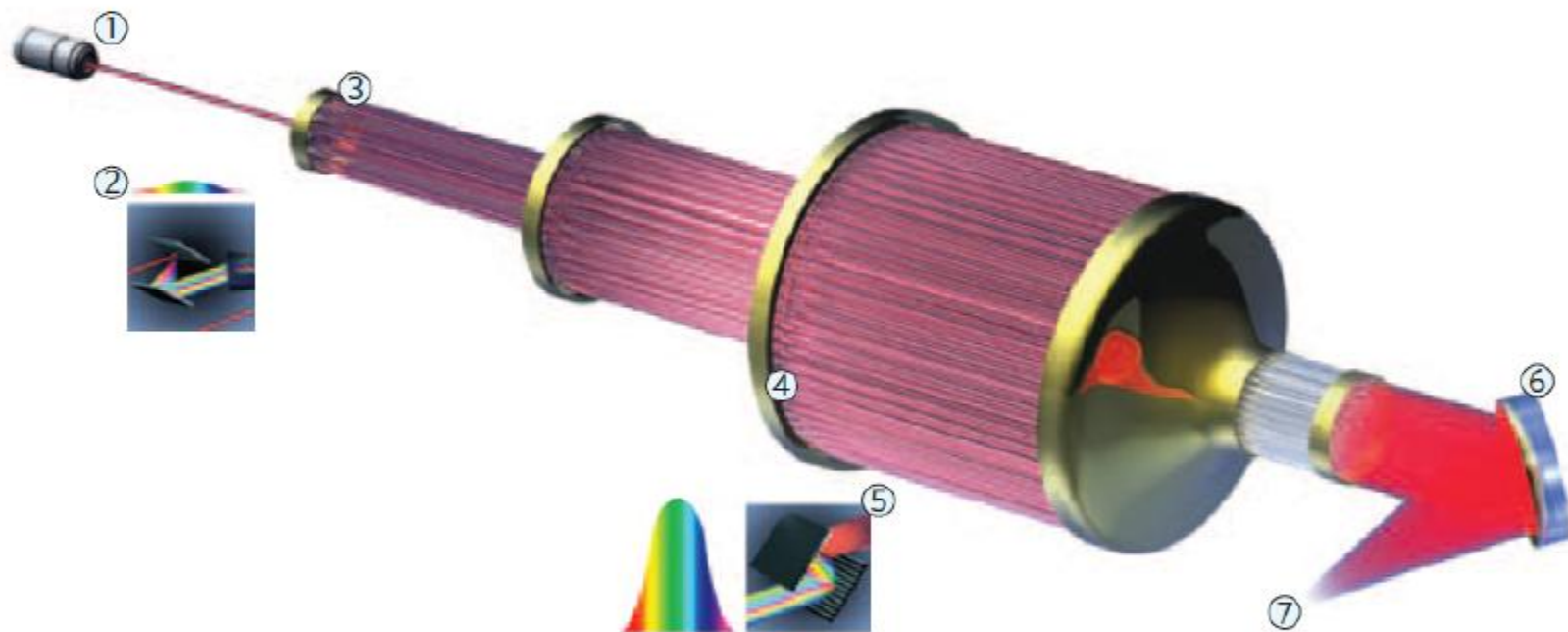
Figure 1 | Principle of a coherent amplifier network. An initial pulse from a seed laser (1) is stretched (2), and split into many fibre channels (3). Each channel is amplified in several stages, with the final stages producing pulses of \sim 1 mJ at a high repetition rate (4). All the channels are combined coherently, compressed (5) and focused (6) to produce a pulse with an energy of >10 J at a repetition rate of \sim 10 kHz (7).
