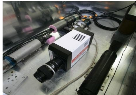
ICCD system and cosmic ray counter
