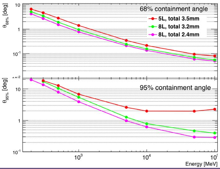
Pattern recognition gets more difficult at high energy for thick converters. Note unconverted  $\gamma$ -ray at high energy can be used
