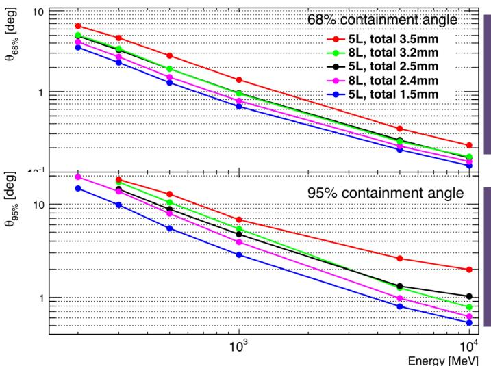
Core resolution depends mainly on MS before the first Si hit, ie. Wthickness of a single layer
