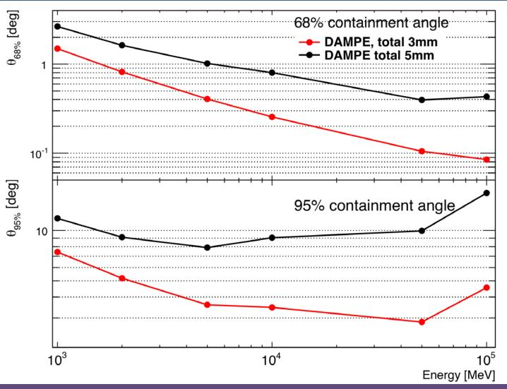
DAMPE is discussing to use 3mm W instead of 5mm Note unconverted  $\gamma$ -ray at high energy can add to efficiency.
